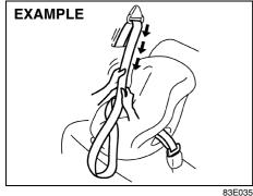
2) Pull all of the remaining webbing out of the retractor. You will hear a click, which means that the emergency locking retractor (ELR) has converted to function as an automatic locking retractor (ALR).
